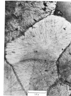
Fig. 5.76 (b) Identical composition heated rapidly to 875^\circ\text{C} and held for 25 min. (From P.E. Doherty in R.M. Fulrath and J.A. Pask, Eds., Ceramic Microstructures , John Wiley and Sons, New York, 1968, pp. 161-185.)
