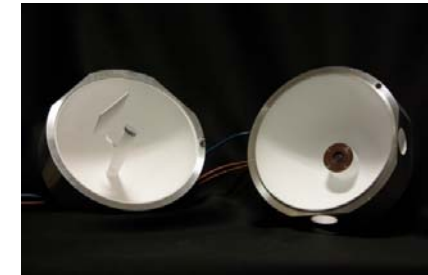
BaSO 4 coated, heatable to 500 K
