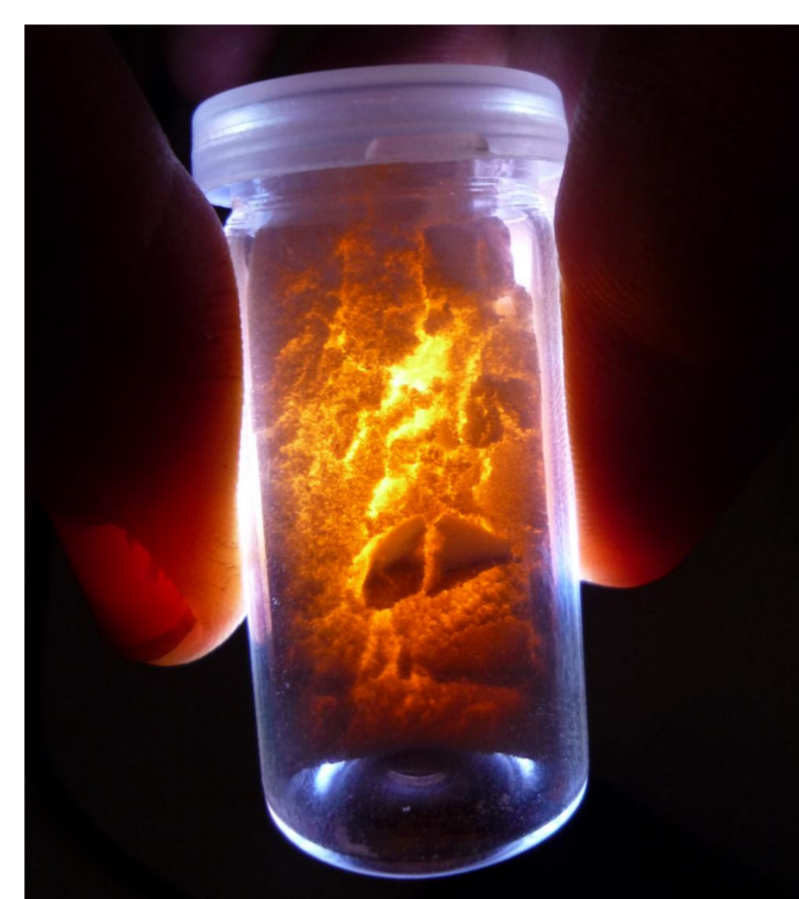
Fig. 4: (Tb 0.8 Eu 0.2 ) 2 Mo 3 O 12 powder irradiated by a smartphone LED
