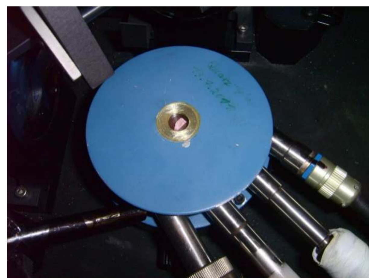
Fig. 1: MicrostatN with connectors for current, temperature detector, vacuum, liquid nitrogen in and gaseous nitrogen out
