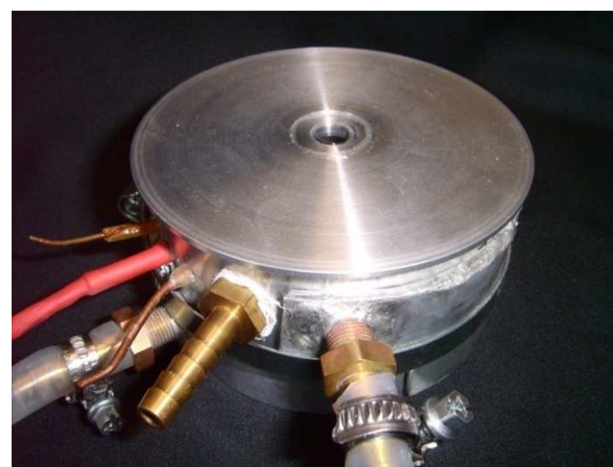
Fig. 2: High temperature sample holder with connectors for current, temperature detector, vacuum and water cooling
