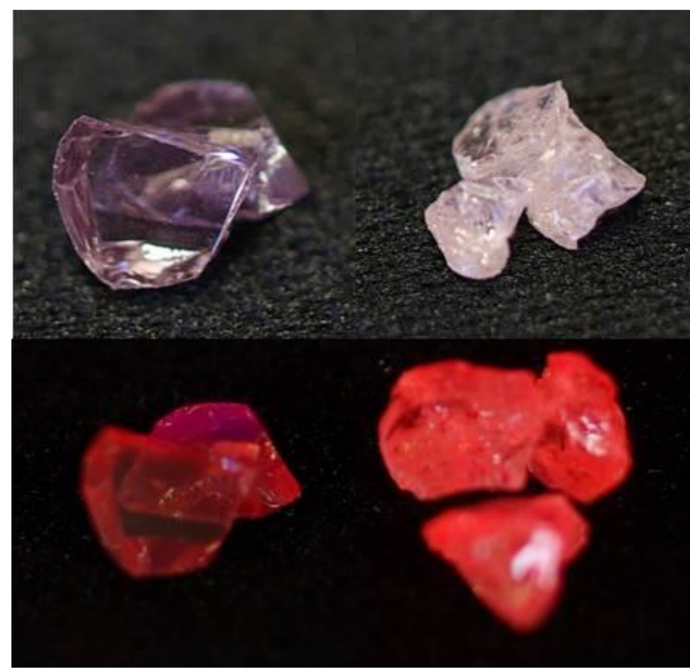
Fig. 1 . LEM crystal fragments of violet LEM (left) and shiny LEM (right) at ambient light (top) and upon excitation at 365 nm (bottom).
